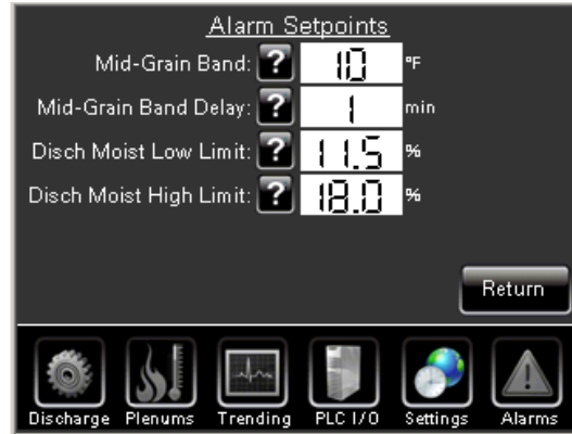
Figure 31: "Alarm Set Point Screen"
